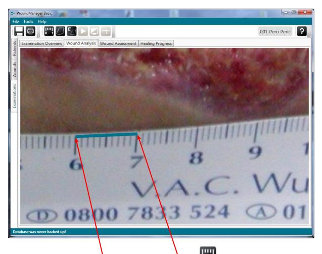
To calibrate the image click at the Calibrate button (), then mark 1 cm distance at the image by clicking the first point, then the second point.
